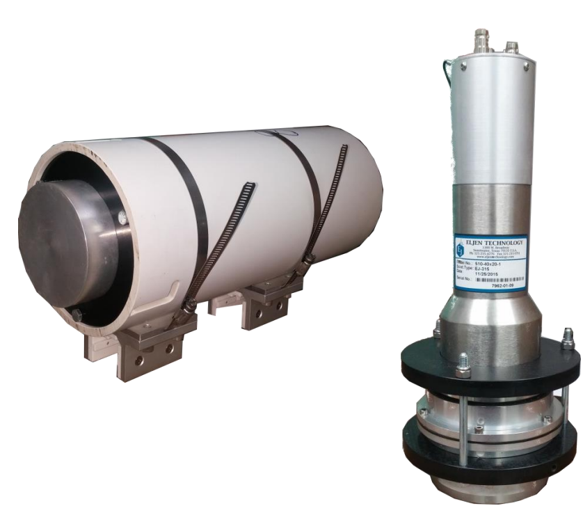
Fig.3: One of CATRiNA detectors with (left) and without (right) mounting case.
