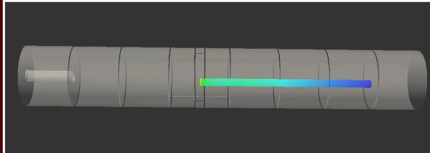
Simulated Penning trap with a single electron track showing the loss of energy due to cyclotron radiation
