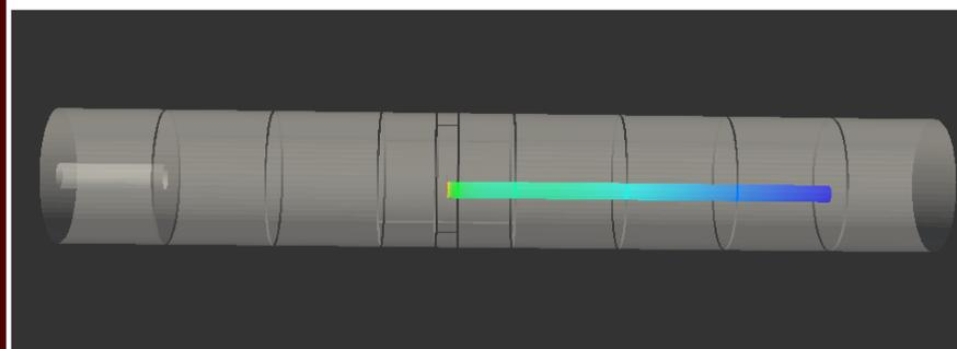
Simulated Penning trap with a single electron track showing the loss of energy due to cyclotron radiation
