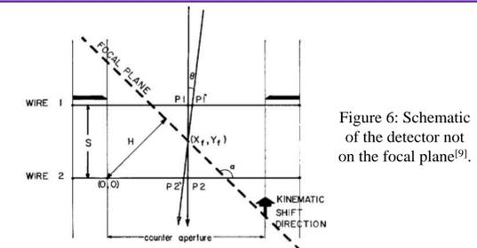
Figure 6: Schematic of the detector not on the focal plane<sup>[9]</sup>.
