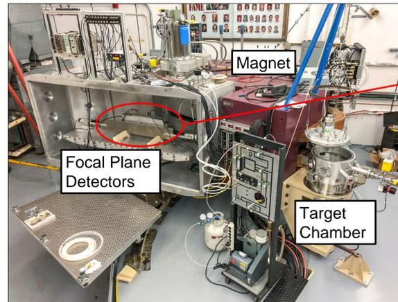
Figure 2: Photo of SE-SPS at FSU with key components labeled.
