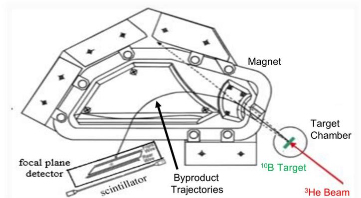
Figure 4: Top down schematic of SE-SPS at FSU showing the particle's trajectories which are governed by the equation  $B\rho = mv/q$ .
