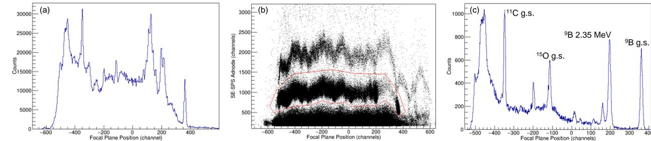
Figure 5: All spectra were generated from a 2 hour long run with a  ${}^{10}\text{B}$  target and the SE-SPS set to 10 degrees. (a) Raw spectra showing all particle counts along the focal plane. (b) Anode channels versus focal plane position where the alpha particles are gated around with a red graphical cut. (c) The graphical cut from 5b is applied to the data shown in 5a and distinct peaks are labeled.
