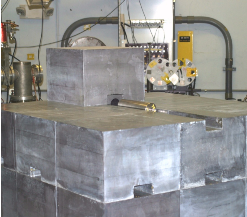
LSDS (partially assembled) and tungsten target
